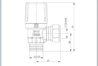
Duco safety valves to protect closed heated and chilled water systems against excessive pressure.
