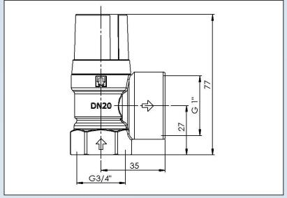
Duco safety valves to protect closed heated and chilled water systems against excessive pressure.
