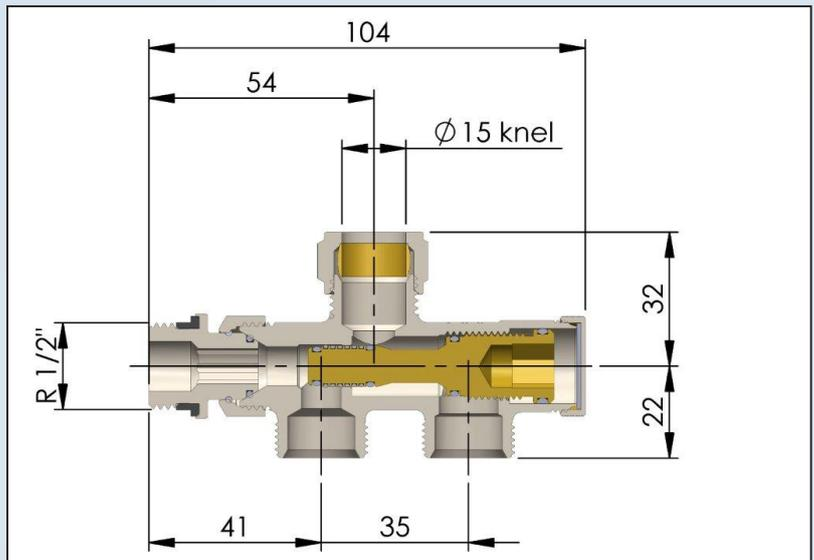
A big advantage of a 2 pipe system is the possibility to adjust the heat (flow) at each radiator independently. By means of the adjustable spindle you can regulate/adjust the flow and also close the supply and return of the valve (in case of removing the radiator).
