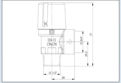
DUCO boilervalves to protect closed potable heated water systems against excessive pressure.
