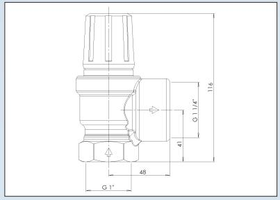
DUCO boilervalves to protect closed potable heated water systems against excessive pressure.
