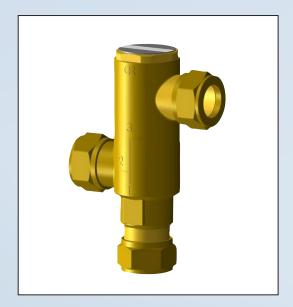
The diverter has to be mounted between the storage tank and the central heating boiler. If the storage tank is able to provide a sufficient amount of hot water, the diverter will lead the water directly to the mixing valve / taps.
