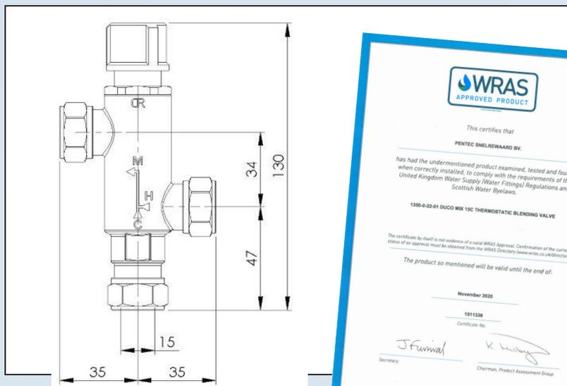
Thermostatic Mixing Valves mix the hot and cold water supplies to ensure constant, safe shower and bath outlet temperatures, preventing scalding.
