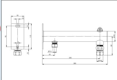
Steel coated console with wall plate to connect expansion vessels up to and including 25 litres to a wall.
