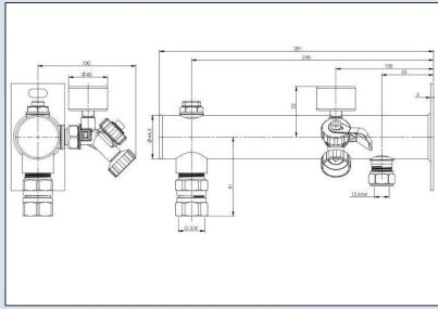
Steel coated console with wall plate to connect expansion vessels up to and including 25 litres to a wall.
