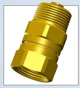
The EVC quick-release coupling makes it easier to connect or disconnect expansionvessels up to and including 25 litres to a pipeline. It is very easy to check, if needed to replace , the correct working of the expansion vessel without draining the entire system.
