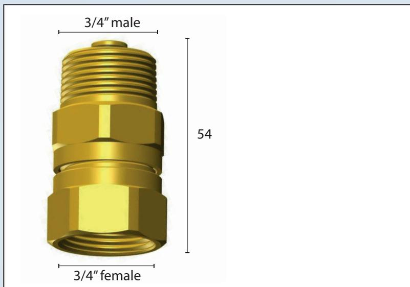
The EVC quick-release coupling makes it easier to connect or disconnect expansion vessels up to and including 25 litres to a pipeline. It is very easy to check, if needed to replace, the correct working of the expansion vessel without draining the entire system.
