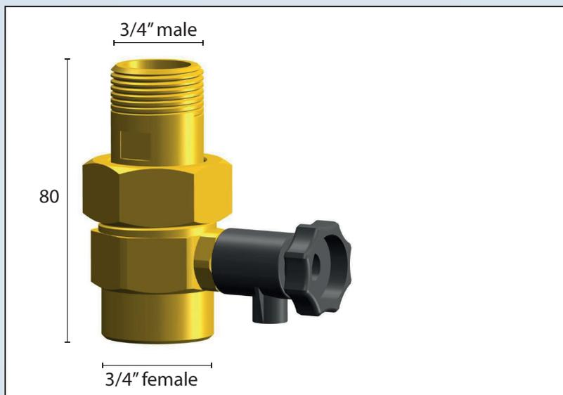
The SU quick-release coupling with drain tap makes it easier to connect or disconnect expansion vessels up to and including 25 litres to a pipeline. It is very easy to check, if needed to replace, the correct working of the expansion vessel without draining the entire system.
